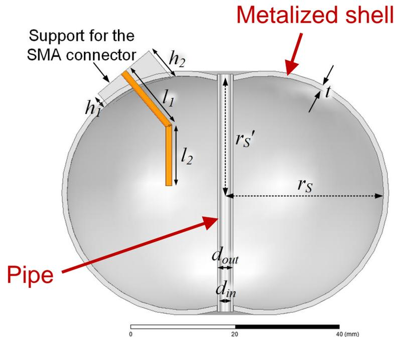
The shape is a **sphere compressed at the poles** (to avoid degenerate modes).
