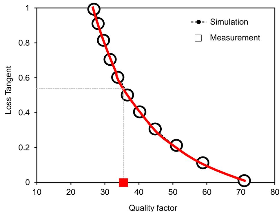
The curve obtained from simulations are used, in conjunction with the **measured quality factor**, to retrieve the loss tangent.
