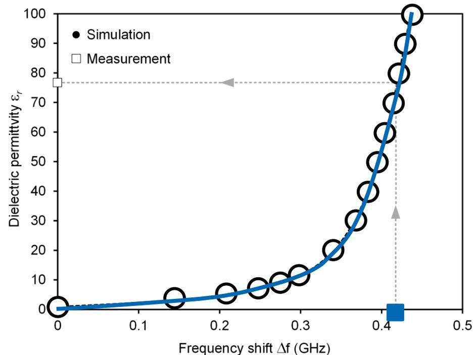
The curve obtained from simulations are used, in conjunction with the **measured frequency shift**, to retrieve the dielectric permittivity.
