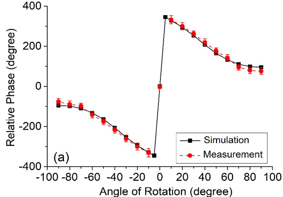
The maximum sensitivity for measuring the angular rotation is found to be a **4.3° change** in the relative phase of the reflection coefficient per **1° of rotation**.
