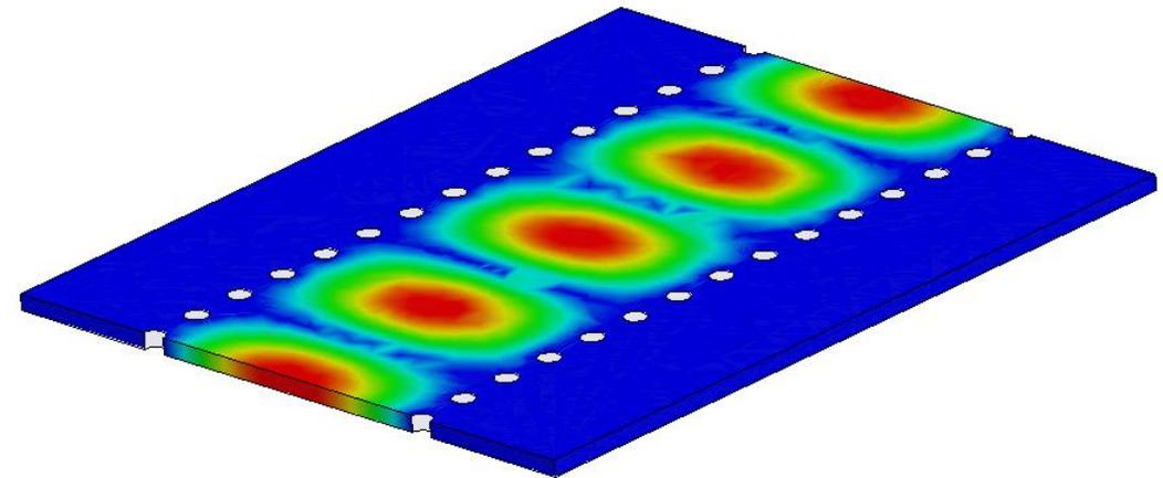
In particular, SIW technology allows implementing **cavity resonators with relatively high quality factor.**
