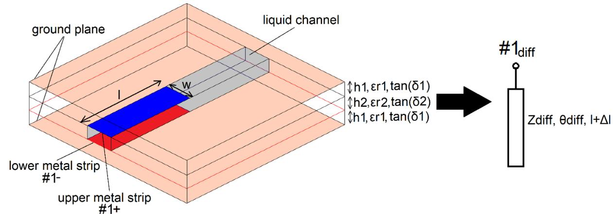
The electrical characteristics of the liquid under test can be obtained from the one-port-differential reflection coefficient, after a proper calibration.
